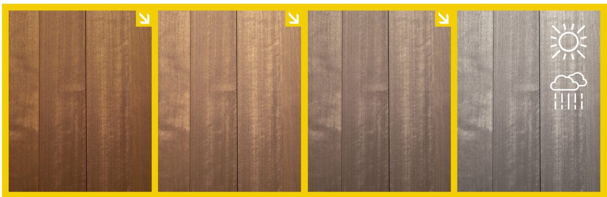
Performance - After Installation | Unoiled wood exposed to UV light
